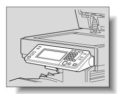
2 To adjust the control panel to an even steeper angle, pull the control panel release lever toward you, and then push down on the control panel.
